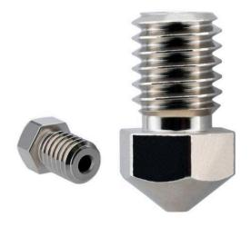
This is RepRap style nozzle, it is made from a 360 brass base material and plated with TwinClad XT coating. TwinClad XT is a nickel composite coating designed for very low friction. It offers one of the lowest coefficient of friction, better than nickel with PTFE co-deposit. This coating is also very hard and abrasion resistant. If you are working with abrasive Carbon Fiber, Stainless Steel, wood filled or any other metal filled filaments, this will greatly improve the life of your nozzle.
